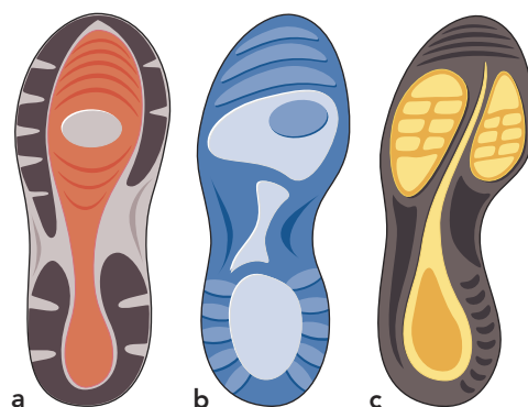
Figure 2.2 Types of lasts: (a) straight, (b) semicurved, and (c) curved.
